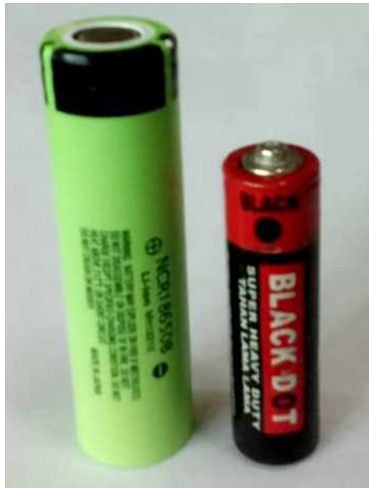
Figure 14 18650 Cylindrical Lithium Battery Cel (left) and AA Battery (right) for comparison
