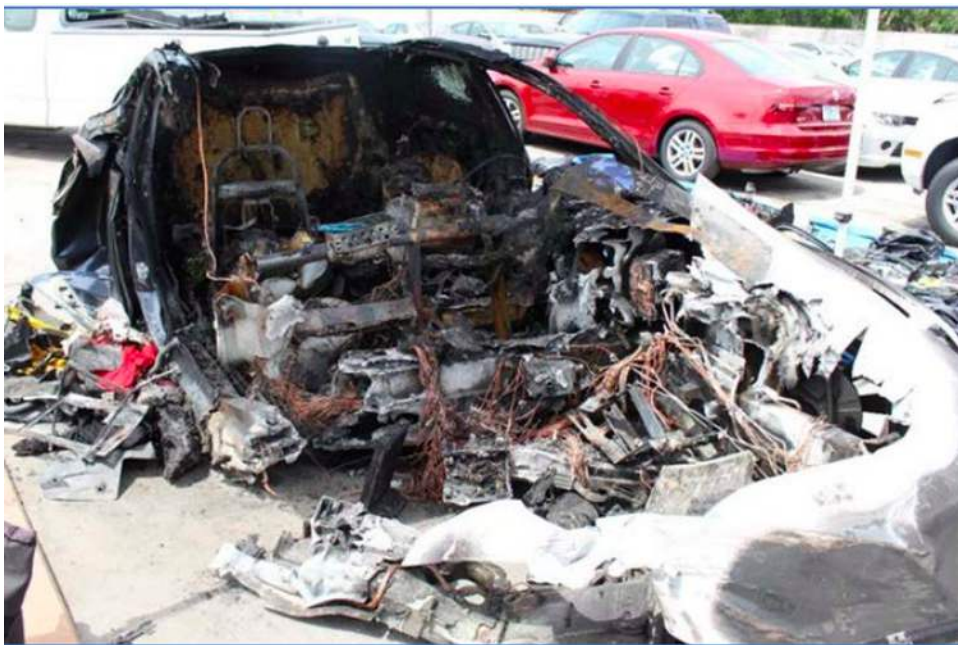
Figure 17 An Electric Vehicle gutted by fire (Chen 2018)
